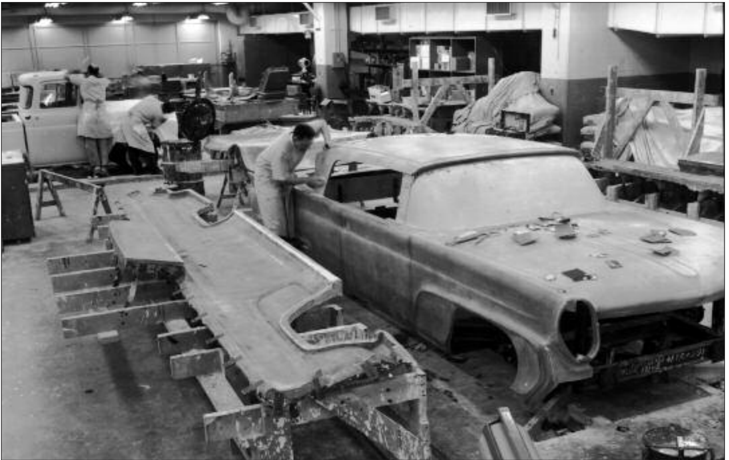
ABOVE After the '58 Lincoln design was finalized and a full-sized clay model was finished and approved, a fiberglass model was built in the Ford shops so an accurate representation of the car could be shown to upper management. BELOW To make the 1958 Mark III clone look different (and more expensive) than the '58 Lincoln, designers added "gorp" to the '58 Lincoln body. Upper management vetoed this proposal. Photos courtesy of the Ford Archives.
