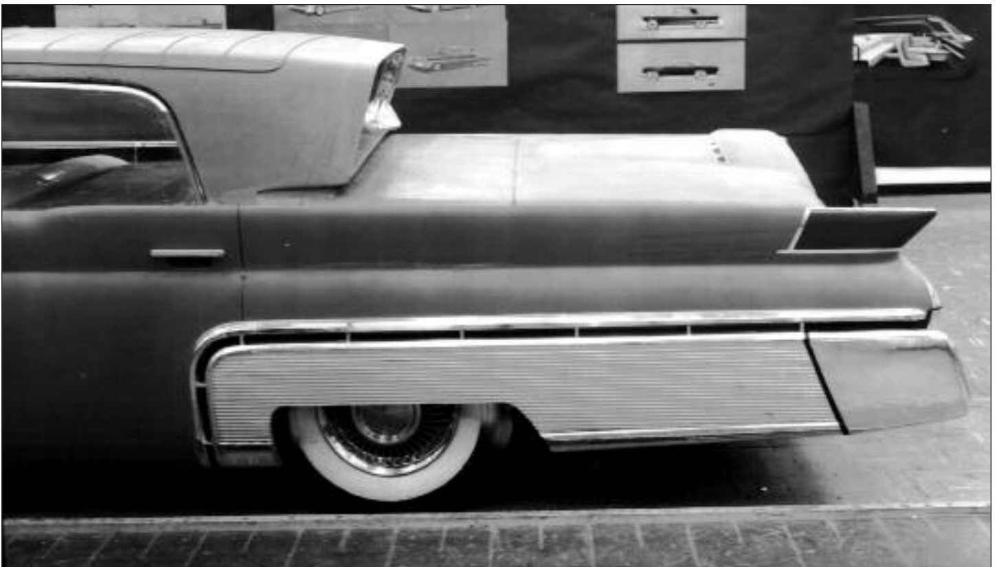
ABOVE After the '58 Lincoln design was finalized and a full-sized clay model was finished and approved, a fiberglass model was built in the Ford shops so an accurate representation of the car could be shown to upper management. BELOW To make the 1958 Mark III clone look different (and more expensive) than the '58 Lincoln, designers added "gorp" to the '58 Lincoln body. Upper management vetoed this proposal. Photos courtesy of the Ford Archives.
